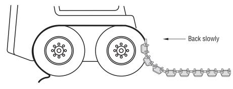
Using a rope or chain, the tracks are easily pulled over the tires by backing the loader slowly.
